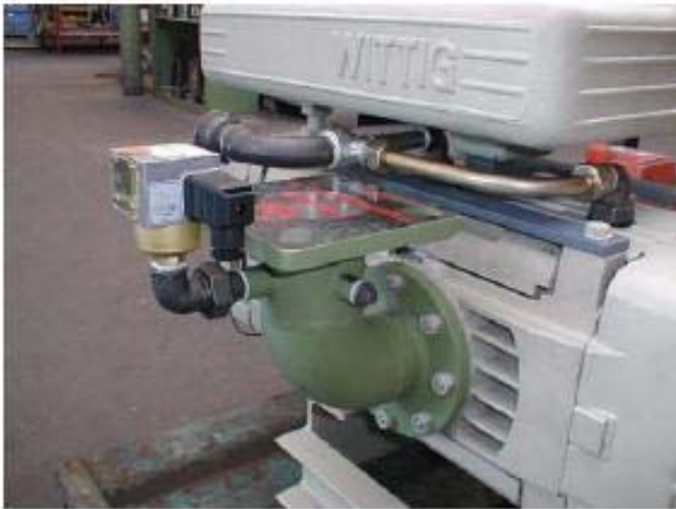
Figure 5.1 Intake manifold and vacuum switches
