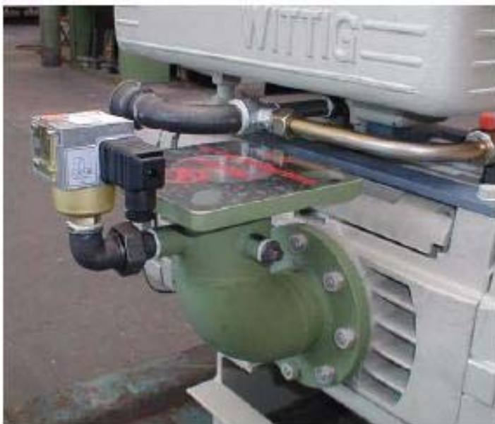
Figure 3.3 With connecting adapters and vacuum switches
